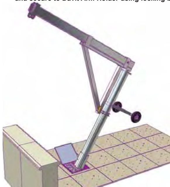
4. Manually raise the arm using hinge pin. Once the arm is the vertical position, insert the second locking pin.
