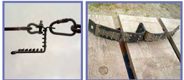
Thaler Energy Absorber (TEA) Before Load Test. Thaler Energy Absorber (TEA) After Load Test
