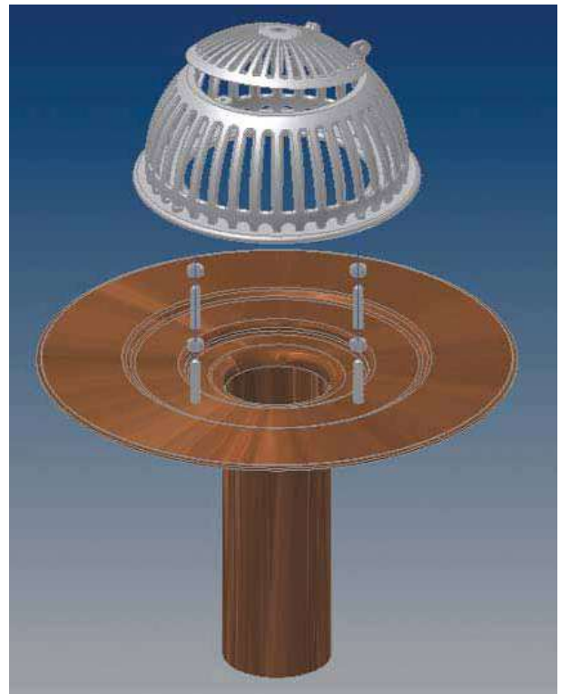
Exploded View Showing four 3/8" (9 mm) mounting bolts welded to four underbody stainless steel reinforcement discs and drain body (flange)
