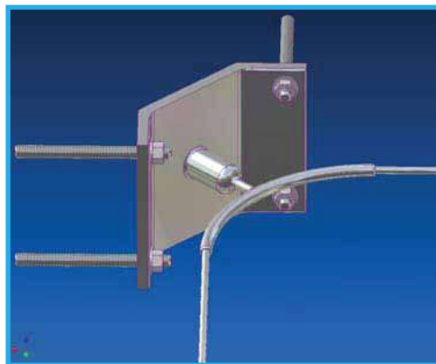
INTERNAL CORNER ANCHOR (90° Angle Illustrated)
